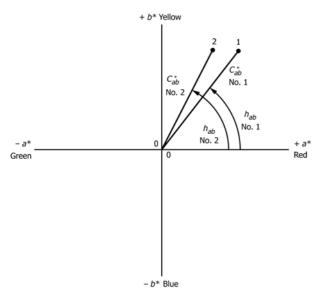
Note 1—Hue angle is measured in degrees starting with  $h_{ab}=0$  in the  $+a^*$  (red) direction and increasing counterclockwise. Chroma is measured as the length of the line from the neutral point  $(a^*=b^*=0)$  to the sample point. Sample Point 2 has a larger value of  $h_{ab}$  than Point 1 and therefore is yellower in hue. Point 2 also has a smaller value of  $C_{ab}$ \* than Point 1 and is therefore lower in chroma or duller.
